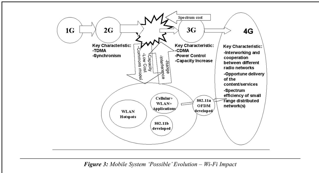
Figure 3: Mobile System 'Possible' Evolution – Wi-Fi Impact
